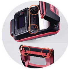
Black Mark and Gap Detection
